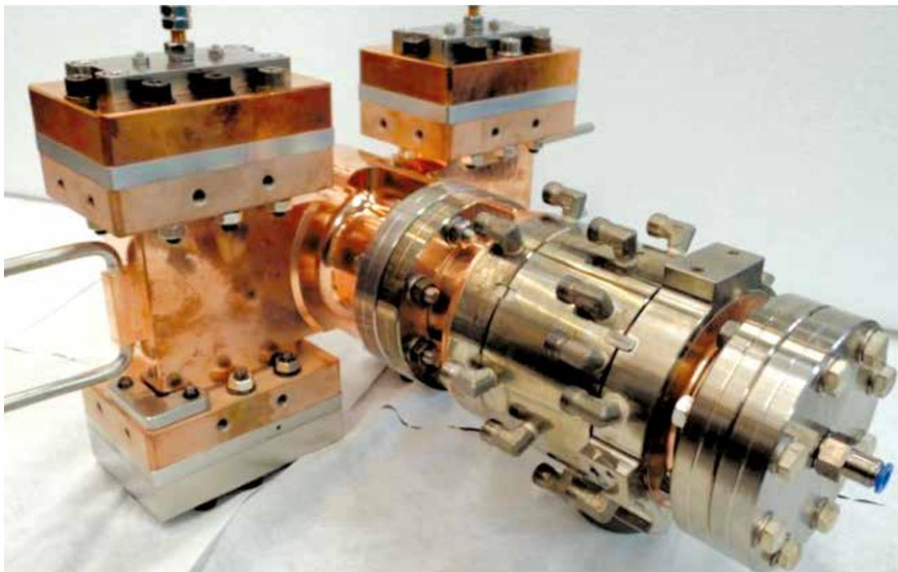
The injector RF cavity upon delivery at Daresbury Laboratory
