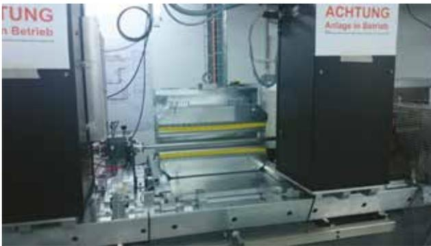
Figure 3: The laser heater undulator, now installed within SwissFEL.
