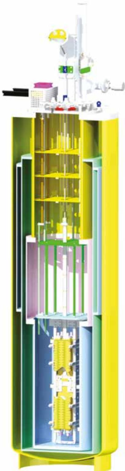
The vertical test cryostat (VTC). The insert (blue section at the bottom) holds the undulator formers.
