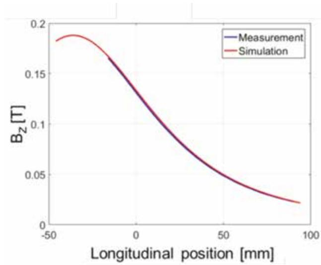
Two solenoid focusing system in the magnet laboratory (left) and comparison of simulated and measured values of the longitudinal magnetic field in the bucking solenoid (right)
