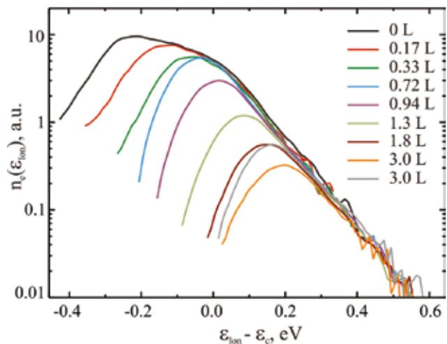
Evolution of the longitudinal energy spread of a GaAsP photocathode with exposure to O<sub>2</sub>.
