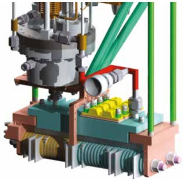
The 'turret' test system used to cool the undulator to  $1.8\text{K}$ . The undulator formers can be seen at the bottom of the picture.
