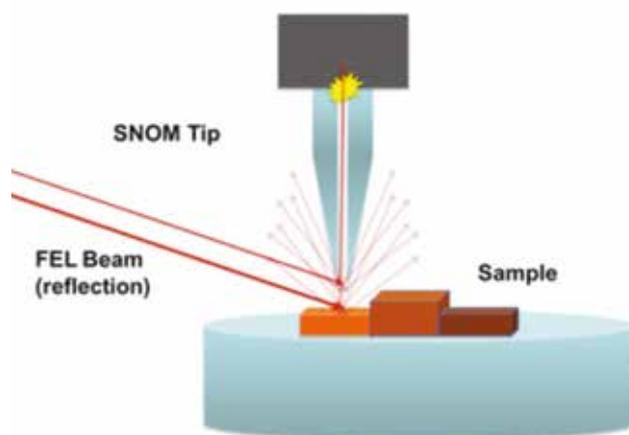
Schematic of the SNOM instrument. The aperture of the SNOM tip is typically 0.1 microns diameter and therefore detects the local absorption of infrared light with sub-micron spatial resolution, below the diffraction limit.
