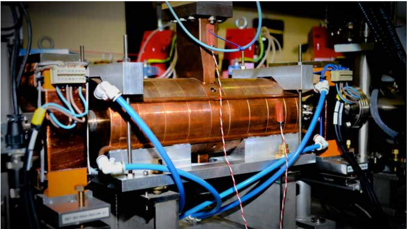
The Transverse Deflecting Cavity installed on VELA.
