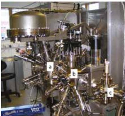
Photocathode preparation system: a - analytical chamber, b-deposition chamber, c- photocathode transport vessel.
