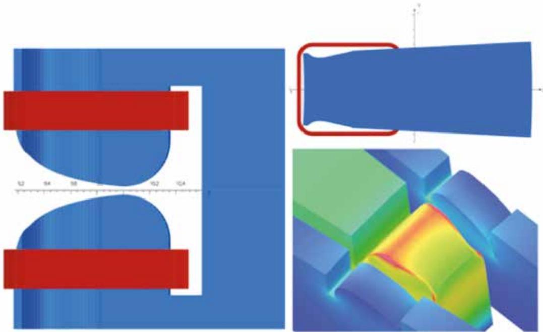
Figure 1: One of the NORMA magnets. (left) Pole area viewed from the side. (right) Magnet viewed from the top, without the clamping plates (top). Pole area with the clamping plates (bottom).
