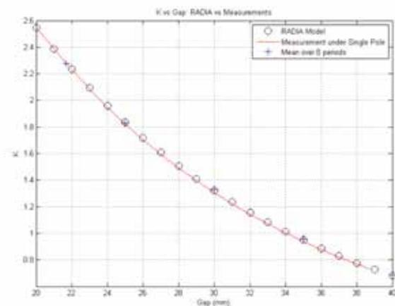
Figure 2: Comparison between the measured and predicted undulator deflection parameter (proportional to the undulator period and on-axis magnetic field strength) as a function of the gap between the undulator arrays
