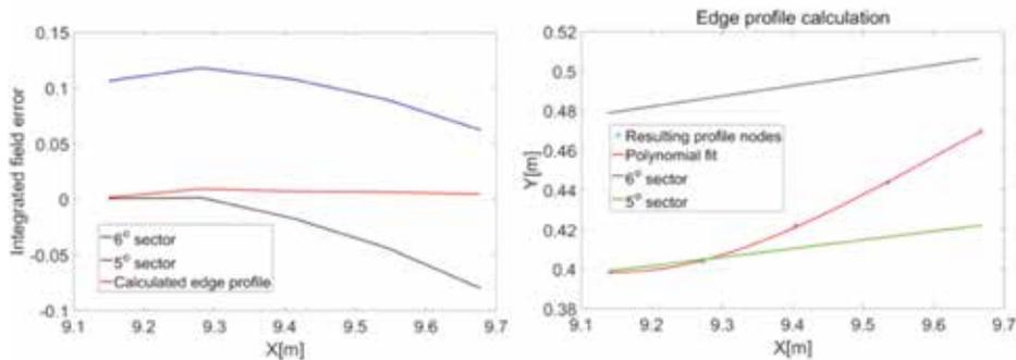
Figure 2: Magnet edge optimization process. (Left) Field errors resulting from three different magnet shapes – a 5-degree, 6-degree sector magnets and from a specially computed edge shape. (Right) The resulting magnet edge shape is shown in comparison with a 5 and 6-degree sector-shaped magnet.
