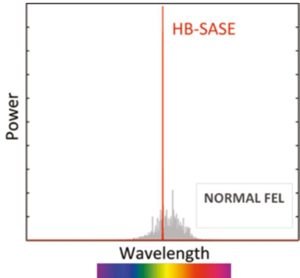
Figure 4: Comparison of the FEL power versus wavelength for a normal FEL (SASE) and High-Brightness SASE. For HB-SASE all the power is at a single wavelength.
