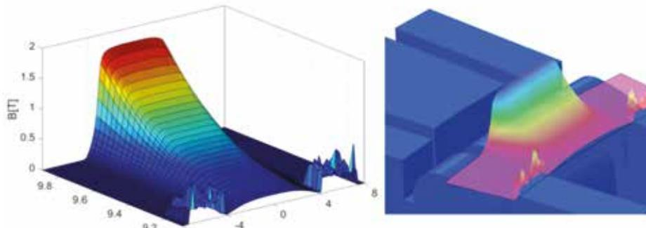
Figure 3: Field generated by a NORMA magnet (Left) A Surface plot of the field in the central symmetry plane. (Right) A surface plot superimposed onto the pole area.
