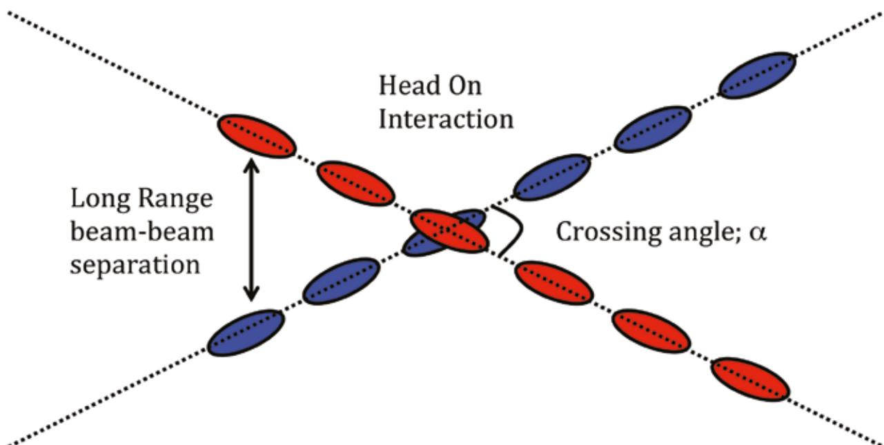
An illustration of the long-range beam-beam interaction versus the standard one is shown (see figure opposite).
