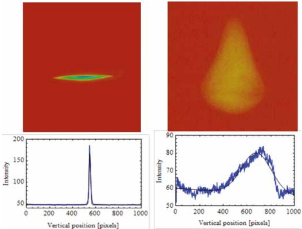
Example images of the beam with the TDC off (left) and with the TDC on (right) giving it the vertical streak in proportion to the electron bunch length. The lower plots show the vertical projections with Gaussian fits.
