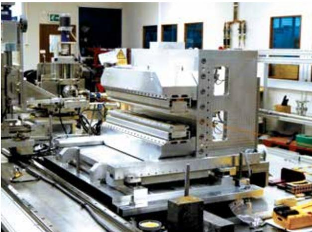
Figure 1: The laser heater undulator being measured at Daresbury.
