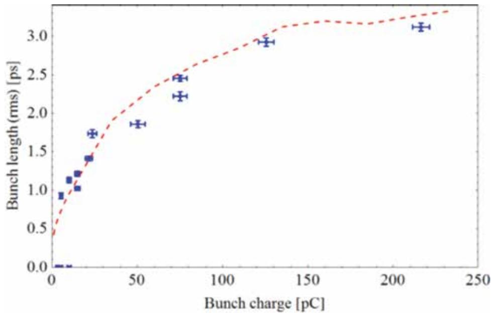
Dependence of the bunch length in VELA as a function of charge, measurements (blue crosses) against simulations (red dotted line).
