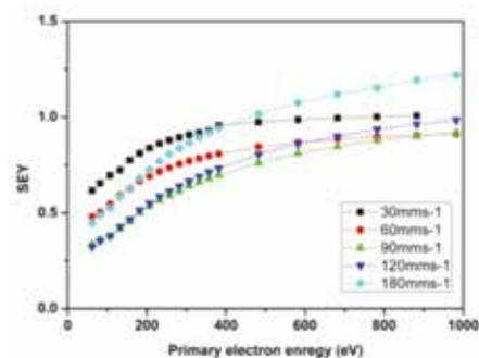
Figure 2: SEY measurement of Cu samples as a function of primary electron energy.
