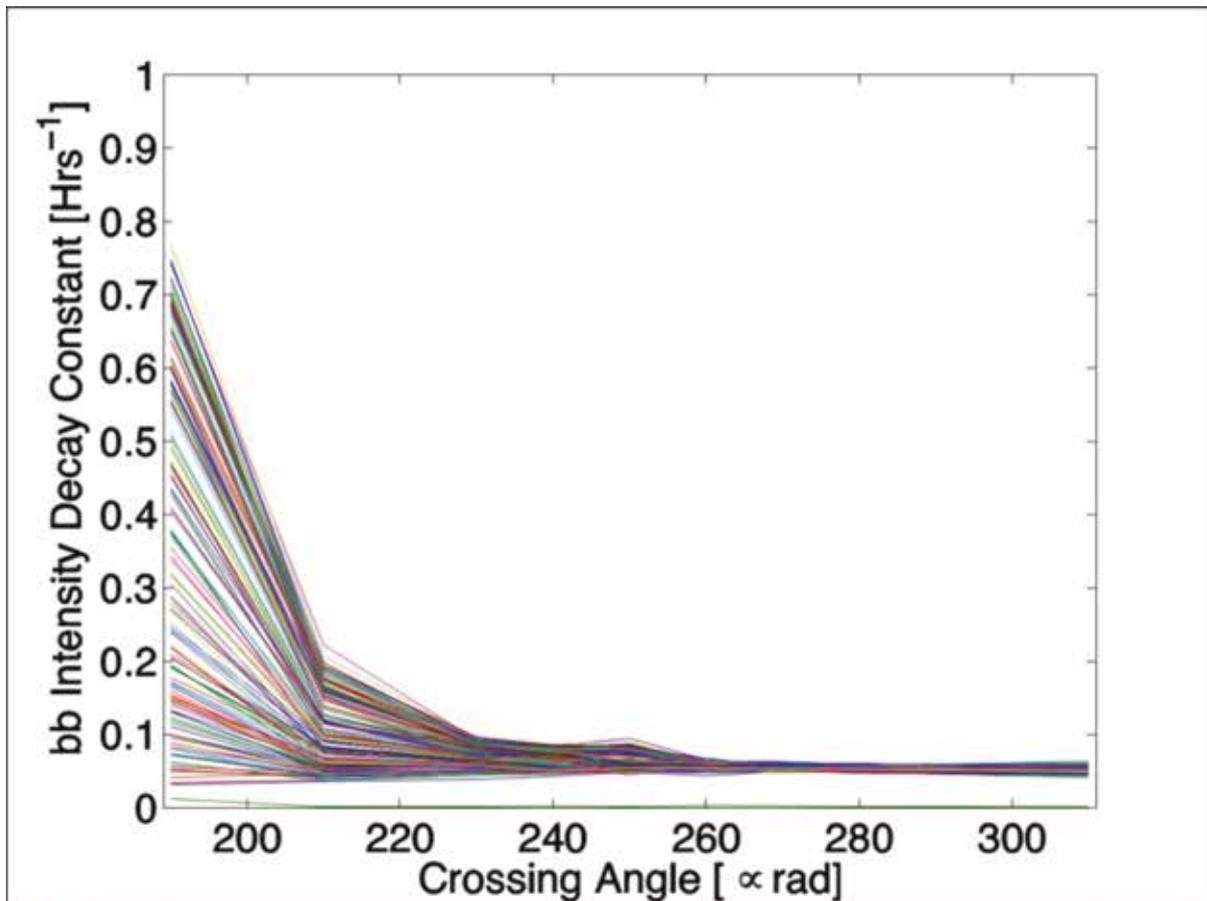
Figure 2: Intensity as a function of crossing angle for the LHC.
