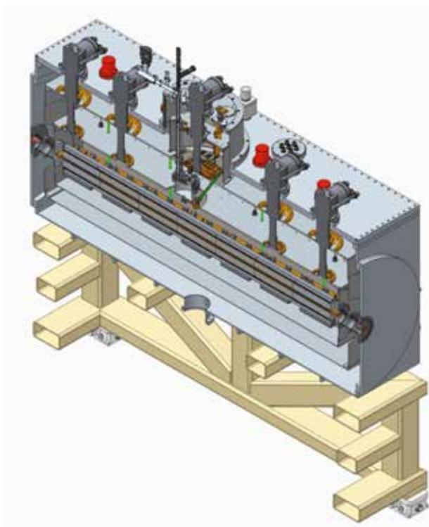
A cutaway view through the cryostat, showing the undulator in the centre. The Diamond beam goes through the vacuum chamber in the centre, shown in orange, and the undulator is split into seven sections surrounding the chamber.
