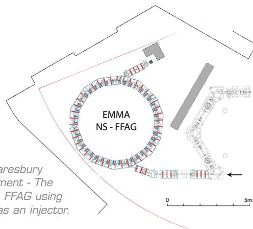
*The Daresbury Experiment - The EMMA FFAG using ERLP as an injector.*
