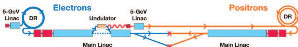
Schematic layout of the International Linear Collider.
