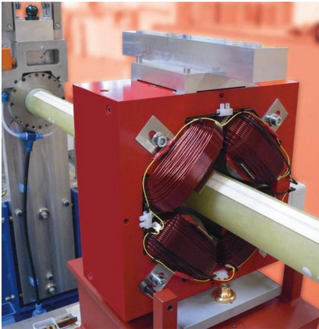
An ERLP quadrupole being measured on a Rotating Coil bench at the Danfysik premises near Copenhagen, Denmark.
