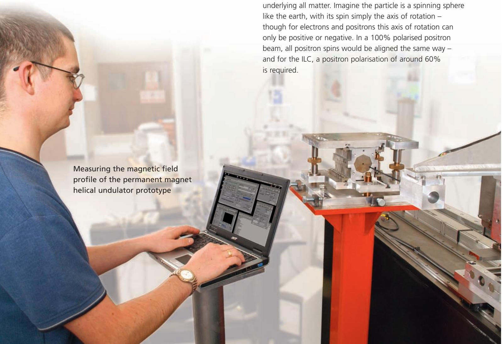
Measuring the magnetic field profile of the permanent magnet helical undulator prototype
