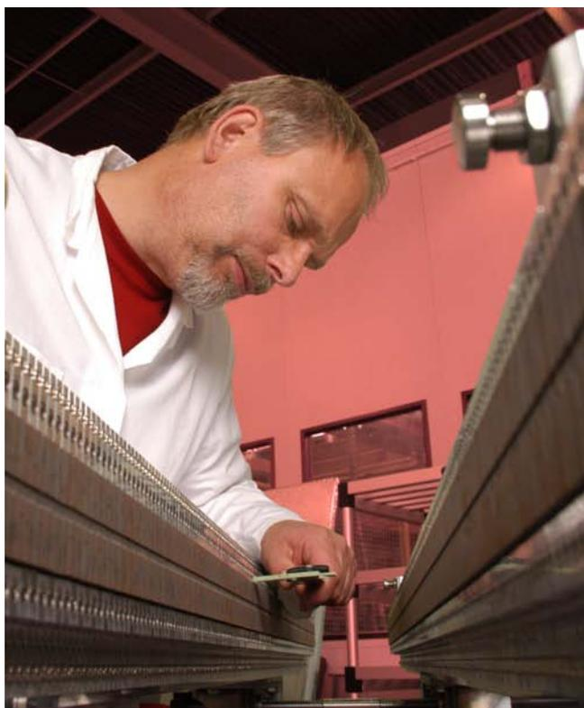
Construction of an ALPHA-X undulator
