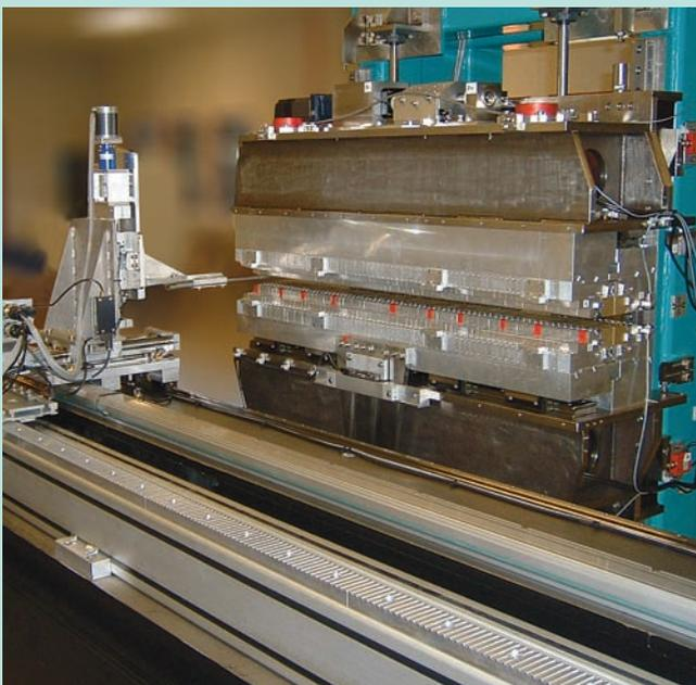
HU56 undergoing Hall probe testing
